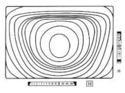
In general, center-weighted average metering is recommended for AE photography. The illustration above shows the metering sensitivity distribution of center-weighted average metering.
